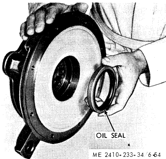
Figure 6-54. Oil seal removal.
