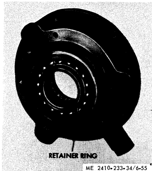
Figure 6-55. Retainer ring removal.
